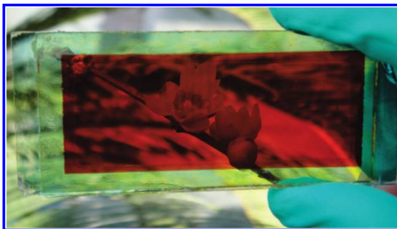
Figure 6. Digital photograph of a large-area bifacially active transparent DSSC fabricated in this work. The cell was sealed with Surlin, and the electrolyte was introduced through a drilled hole on the counter electrode.
