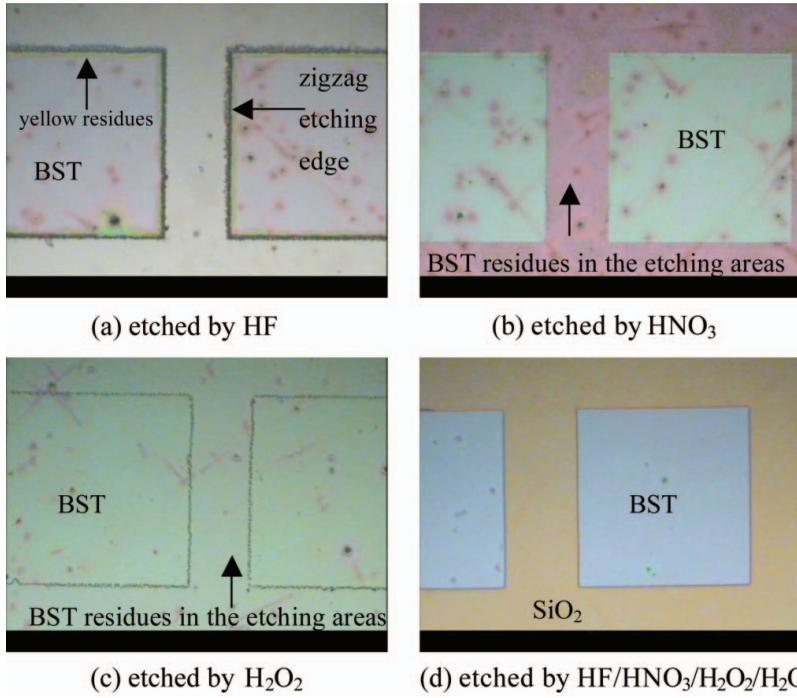
Figure 1. Metallographs of BST thin films etched by different etchant. (See Color Plate XXVII)
