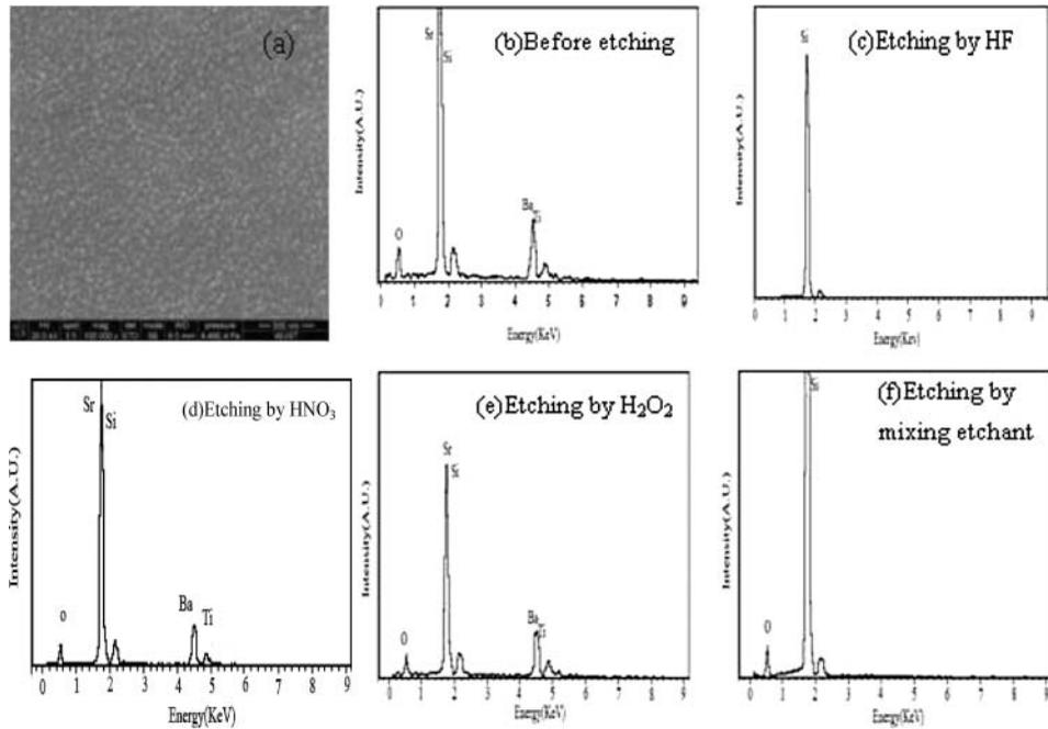
Figure 2. SEM with EDS analysis of BST films annealed at 700°C.
