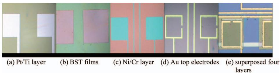
**Figure 6.** The metallographs of the detector arrays. (See Color Plate XXX)
