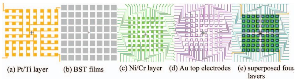
**Figure 5.** The designed mask patterns of the detector arrays. (See Color Plate XXIX)
